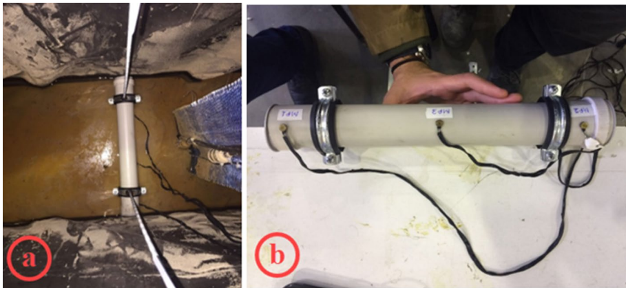
Fig. 7 a Free pipe model with attached potentiometers, and b fixed pipe model with attached load cells
