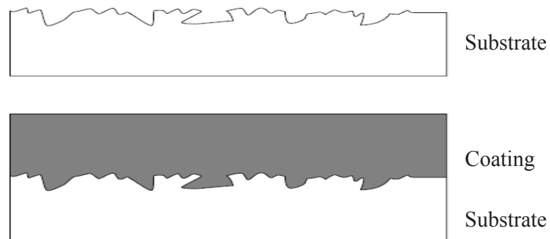
Figure 6. Illustration of mechanical interaction between the coating and substrate 2
