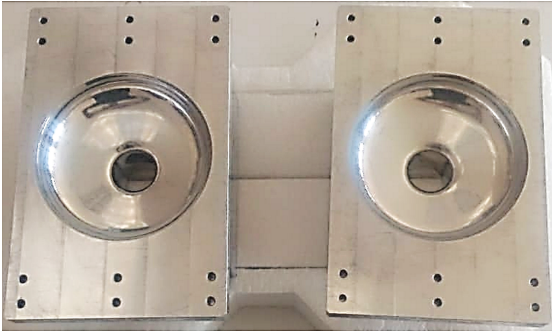
Figure 4.16. Image of 2 Separate Half-Cells of a 1-Cell Elliptical Cavity
