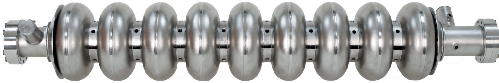
Figure 1.3. 9-Cell Elliptical Cavity (Source:Vostrikov, 2015)
