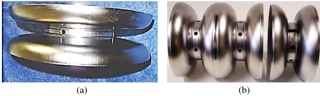
Figure 1.5. Fabricated Mid Dumbbells (a) Cavity at JLAB (b) TESLA Cavity (Source: Delayen, 2008)
