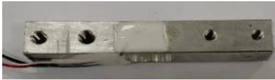
Figure 4.1. Demonstration of load cell to measure the weight
