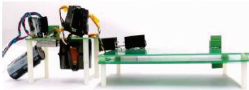
Figure 1.9. Prototype of 30 W capacitive WPT system (Source: Chang et al., 2015)
