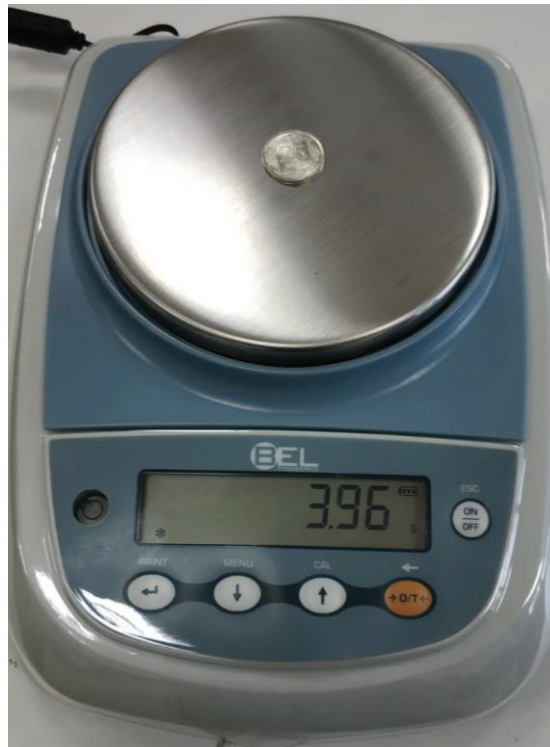
Figure 5.4. The measured mass of 0.25 TL coin by precision laboratory scale
