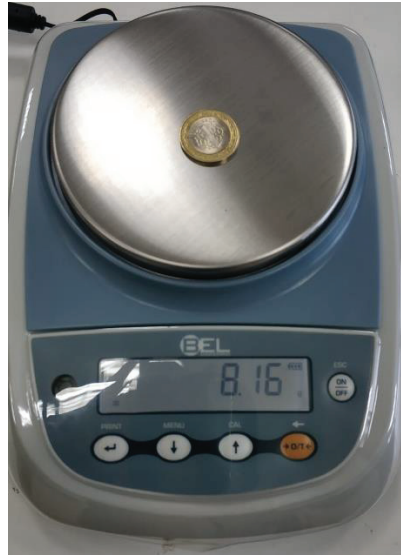
Figure 5.1. The measured mass of 1 TL coin by precision laboratory scale
