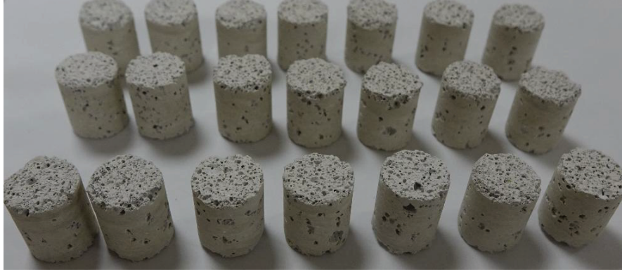
Figure 3.6. The picture of core-drilled G406 samples after cleaning with pressurized air
