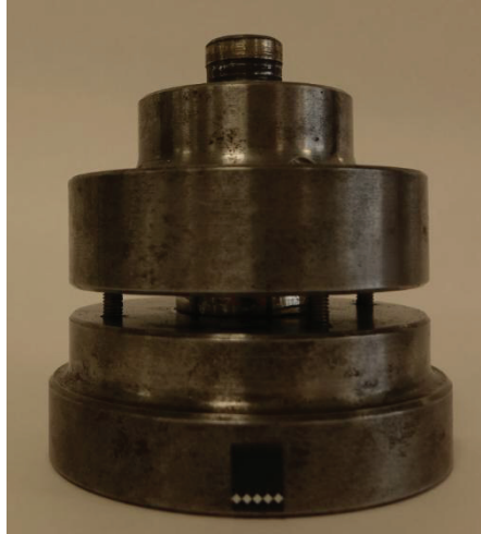
Figure 3.8. Axially aligned pin-ball compression upper platen
