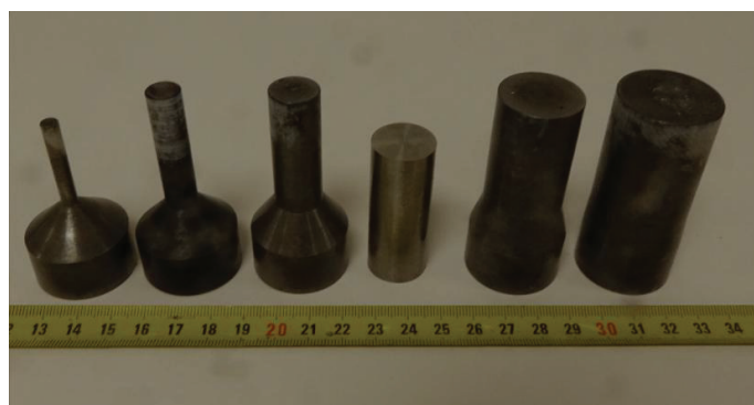
Figure 3.9. 5, 10, 15, 20, 25 and 30 mm diameter indenters
