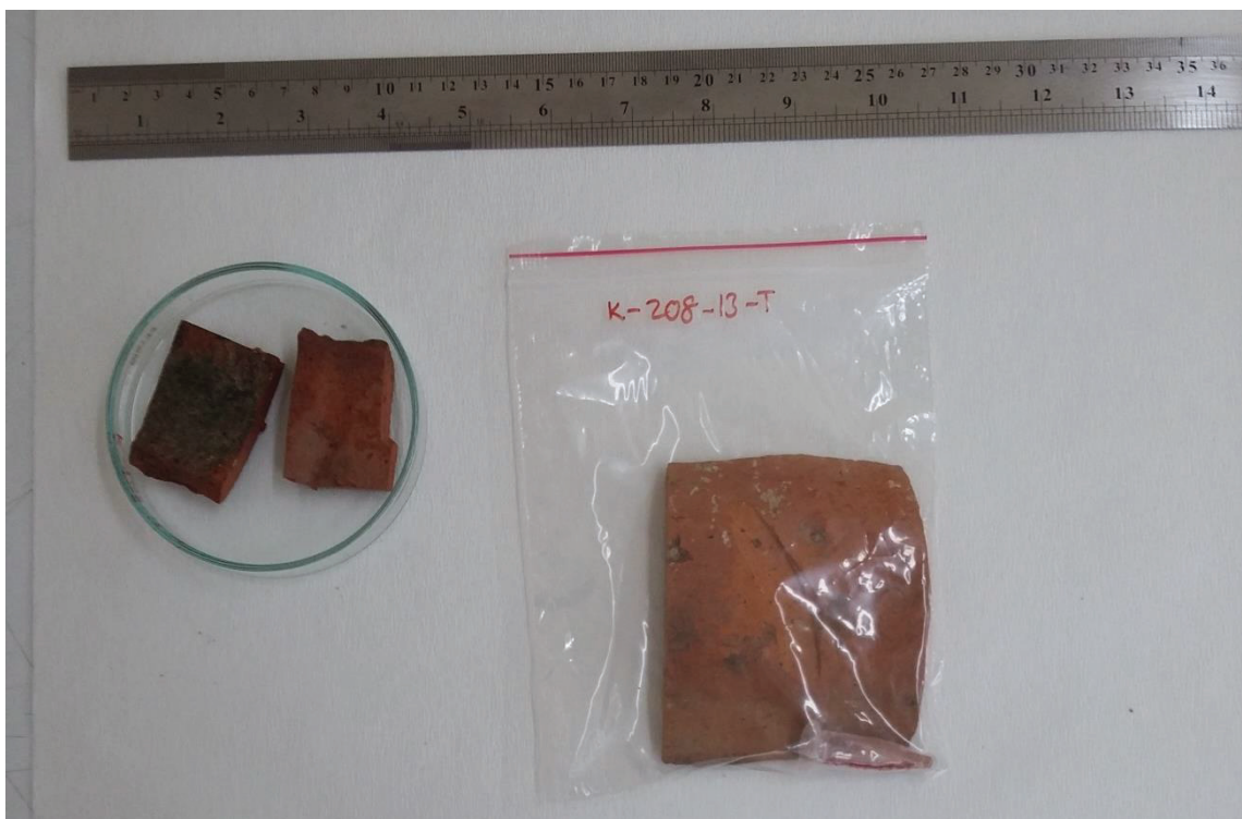
Figure 190. Material sample K-208-13-T processed for thermophysical measurements
