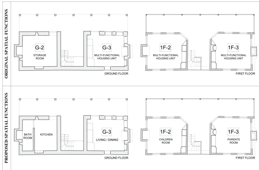
Figure 64. Proposed spatial functions for the model of Sönmezer House in comparison to the original utilization
