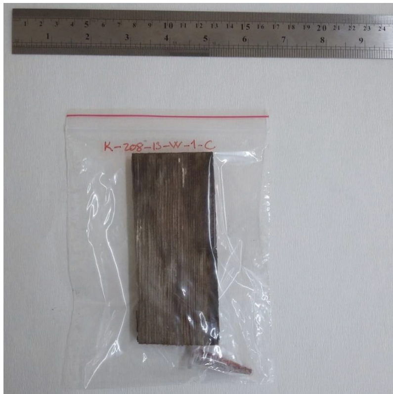
Figure 192. Material sample K-208-13-W-1-C processed for thermophysical measurements
