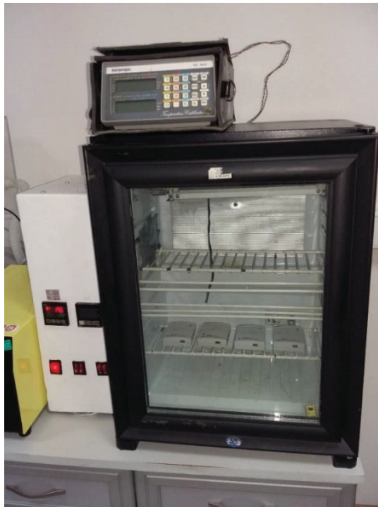
Figure 8. Chamber for temperature calibration tests
