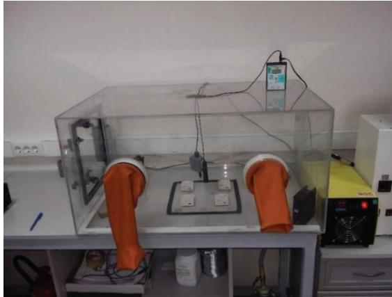
Figure 9. Chamber for relative humidity calibration tests
