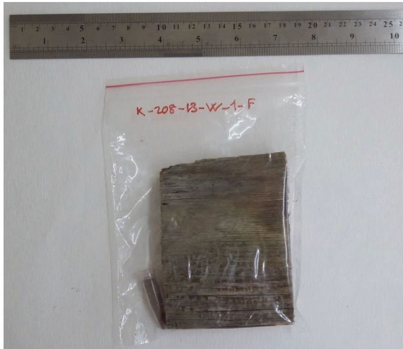
Figure 191. Material sample K-208-13-W-1-F processed for thermophysical measurements
