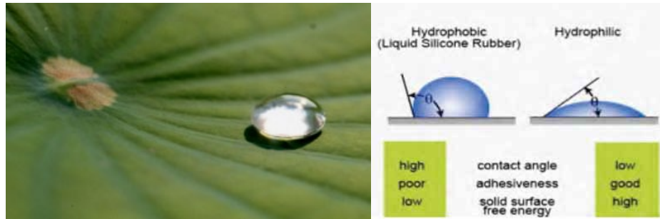
Figure 26. Water droplet and solid surface energy diagram by Ensikat, Ditshe-Kuru, Neinhuis, & Barthlott (2011)
