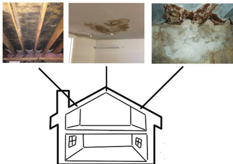
Figure 4. Damages are on the building floor due to moisture accumulation
