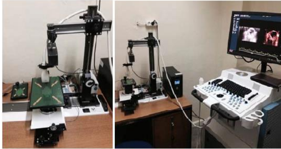
Figure 3.8. The Vevo 2100 ultrasonographic system, 3-D transducer positioning platform and the experimental animal stabilization panel.
