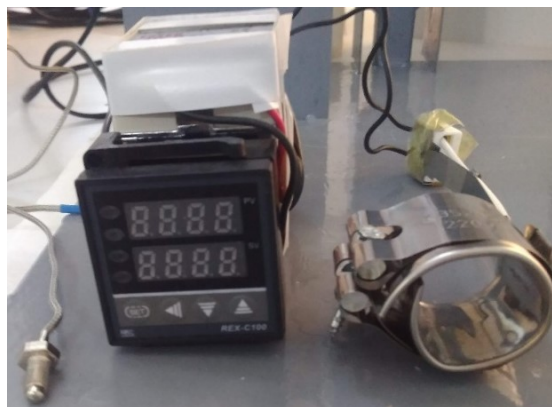
Figure 2.5. The heat controller.
