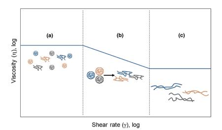
**Figure 1** Schematic representation of the viscosity-shear rate behavior of hydrocolloid polymer solutions above C\* (adapted from Khatibi *et al.*, 2016).
