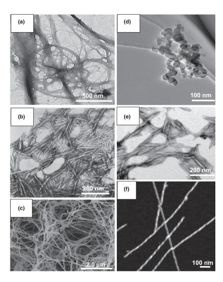
Figure 2 TEM images of (a) MFC and (b) CNCs; SEM micrographs of (c) BC; (d) SNCs (reproduced with permission from Elsevier Ltd [Wang et al., 2010; ]); (e) chitin nanocrystals (reproduced with permission from Elsevier Ltd [Wang et al., 2012]); (f) AFM image of amyloid fibrils with twisted ribbon morphology (reproduced with permission from Elsevier Ltd [Adamcik & Mezzenga, 2012]).
