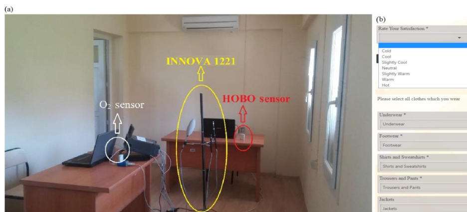
Figure 2. (a) Location of the sensors and (b) screenshots of mobile application interface
