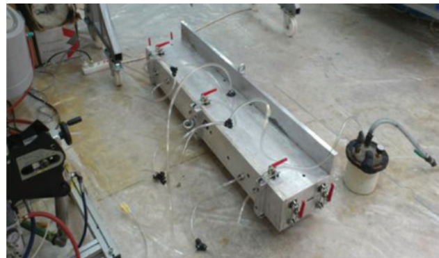
Figure 12: Manufacturing setup for the composite-based mono-leaf spring.
