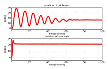
Fig. 6. Angular pitch (top) and yaw (bottom) positions for lag compensators of the form  $10\left(\frac{s+0.1}{s+0.01}\right)$  and  $10\left(\frac{s+0.1}{s+0.001}\right)$  applied on the main and tail motors, respectively.
