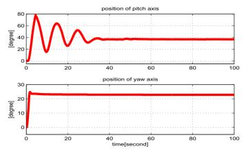
Fig. 5. Angular pitch (top) and yaw (bottom) positions for proportional controllers with gains 10 and 3000 for the main and tail motors, respectively.
