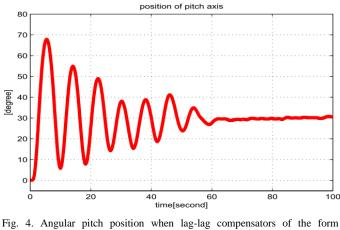
Fig. 4. Angular pitch position when hag-lag compensators of the form  $10\left(\frac{s+0.1}{s+0.01}\right)^2$  was applied on the main motor.
