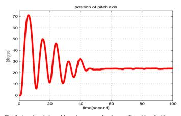
Fig. 2. Angular pitch position when proportional controller with gain 10 was applied on the main motor.
