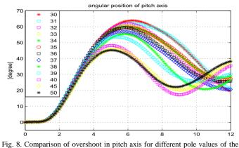
Fig. 8. Comparison of overshoot in pitch axis for different pole values of the lead compensator.
