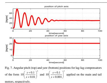
In view of the experimental results obtained testing the twin rotor system in our laboratory, the lag type compensation significantly improves the steady state error when compared with proportional controllers.
