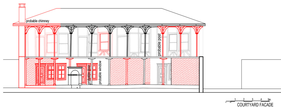
Fig. 13. Reconstructions of hayat elevations: (a) Kerimağa House, Birgi ; and (b) Eker House, Kirkağaç .
