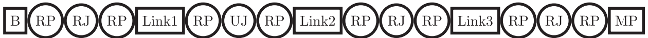
Fig. 15. Illustration of connections in ANSYS. RP: Remote Point, RJ: Revolute Joint, UJ: Universal Joint, B: Base, MP: Mobile Platform.
