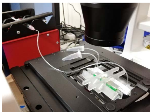
Fig. 6. The sorting setup consisting of the magnetic levitation platform, the syringe pump and the microscope.
