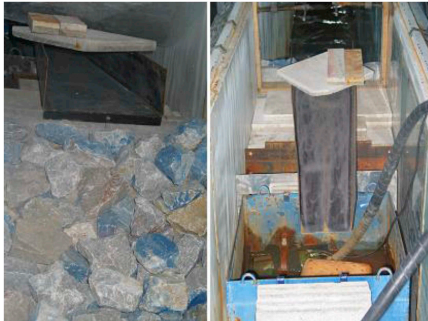
Fig. 4. Overtopping measuring system.
