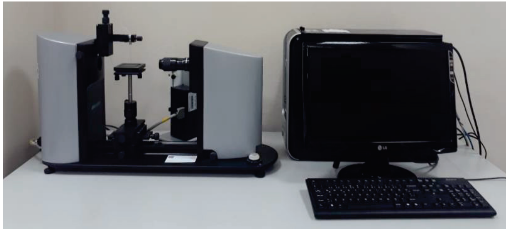
Figure 3.9. Contact angle measurement instrument in IZTECH
