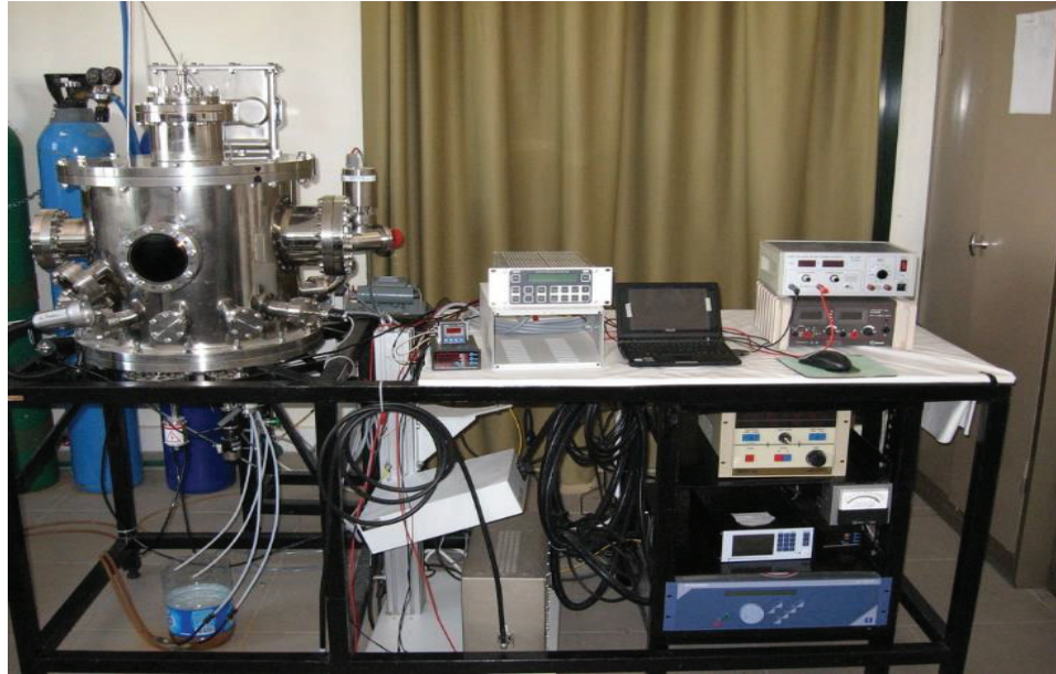
Figure 3.1. The schematic representation of D.C. Magnetron Sputtering System
