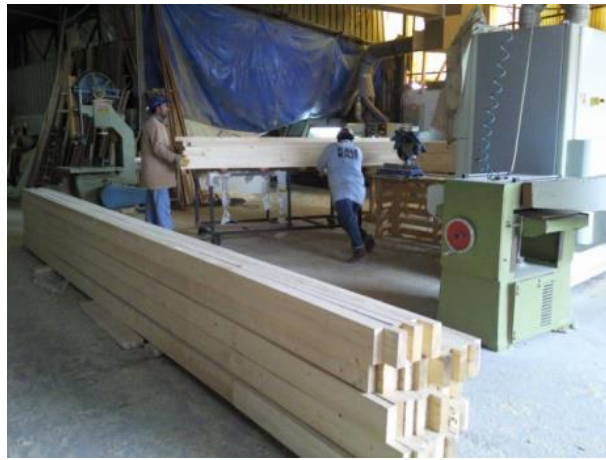
Figure 5.23. Manufacture of Laminated Wood Pieces
