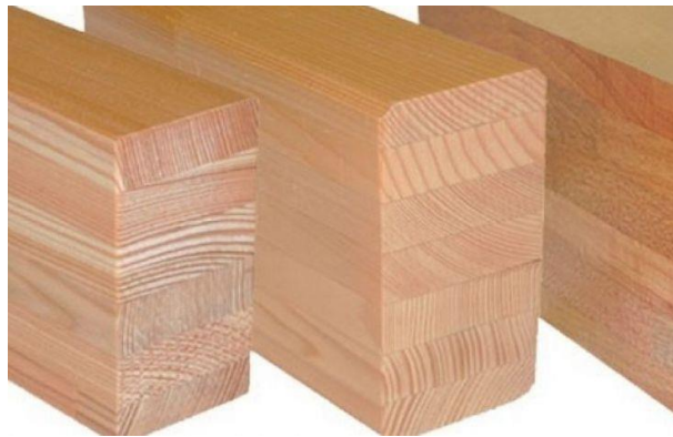
Figure 4. 16. Glue Laminated Timber 52
