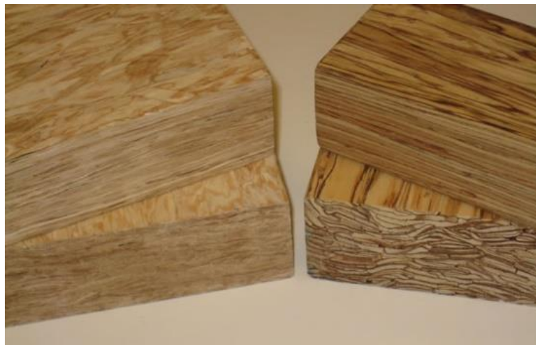
Figure 4. 17. Oriented Strand Lumber 53
