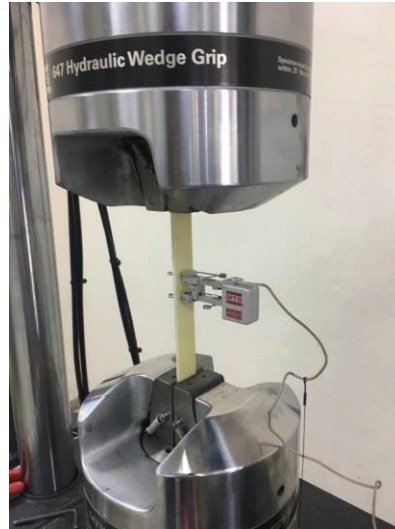
Figure 3.3. Tensile test specimen during test
