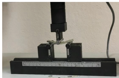
Figure 3.4. Flexural test specimen during test
