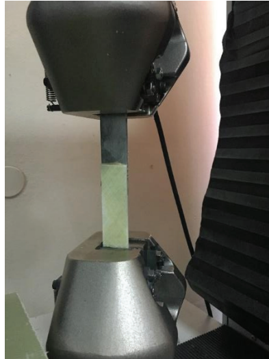
Figure 3.10. Single lap shear test specimen during test
