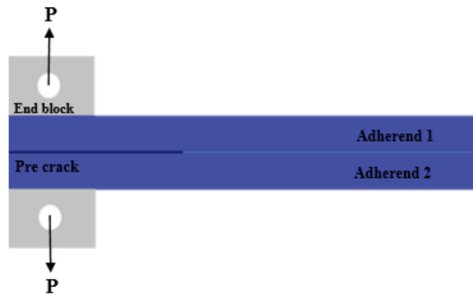
Figure 2.7. Schematic of DCB test specimen under tensile loading
