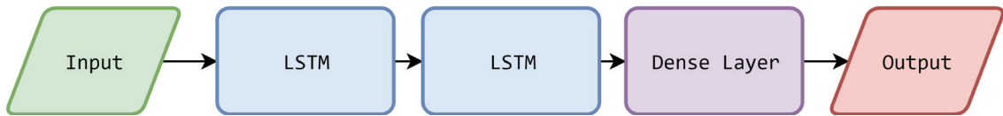
Figure 4.5. The foundational model is a simple 2-layer LSTM network followed by a single dense layer having size as the number of output features.
