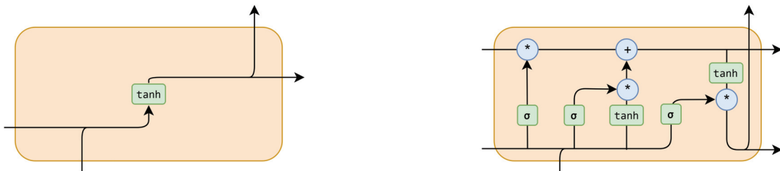
Figure 3.10. While RNN node (left) has only a \tanh activation gate in its data flow, LSTM node (right) also has a cell-state which can be updated or flushed when needed.
