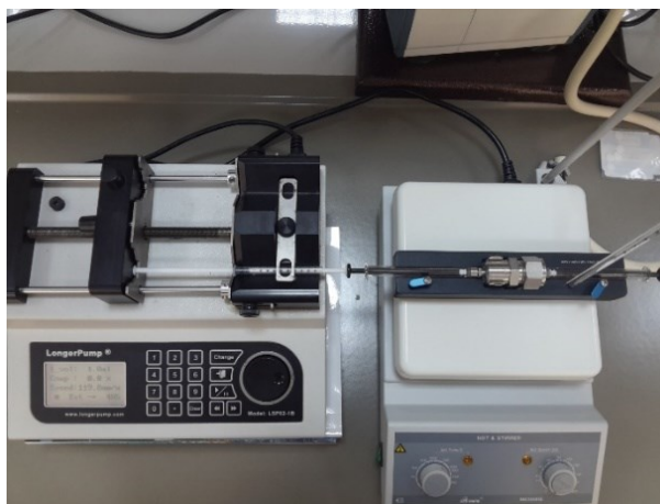
Figure 4.2. Extrusion set-up with syringe pump (in left hand-side) and mini-extruder (in right hand-side, on the top of heater)
