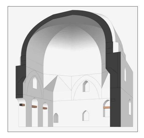
Figure 5.12. Schematic representation of new lintel system in walls
