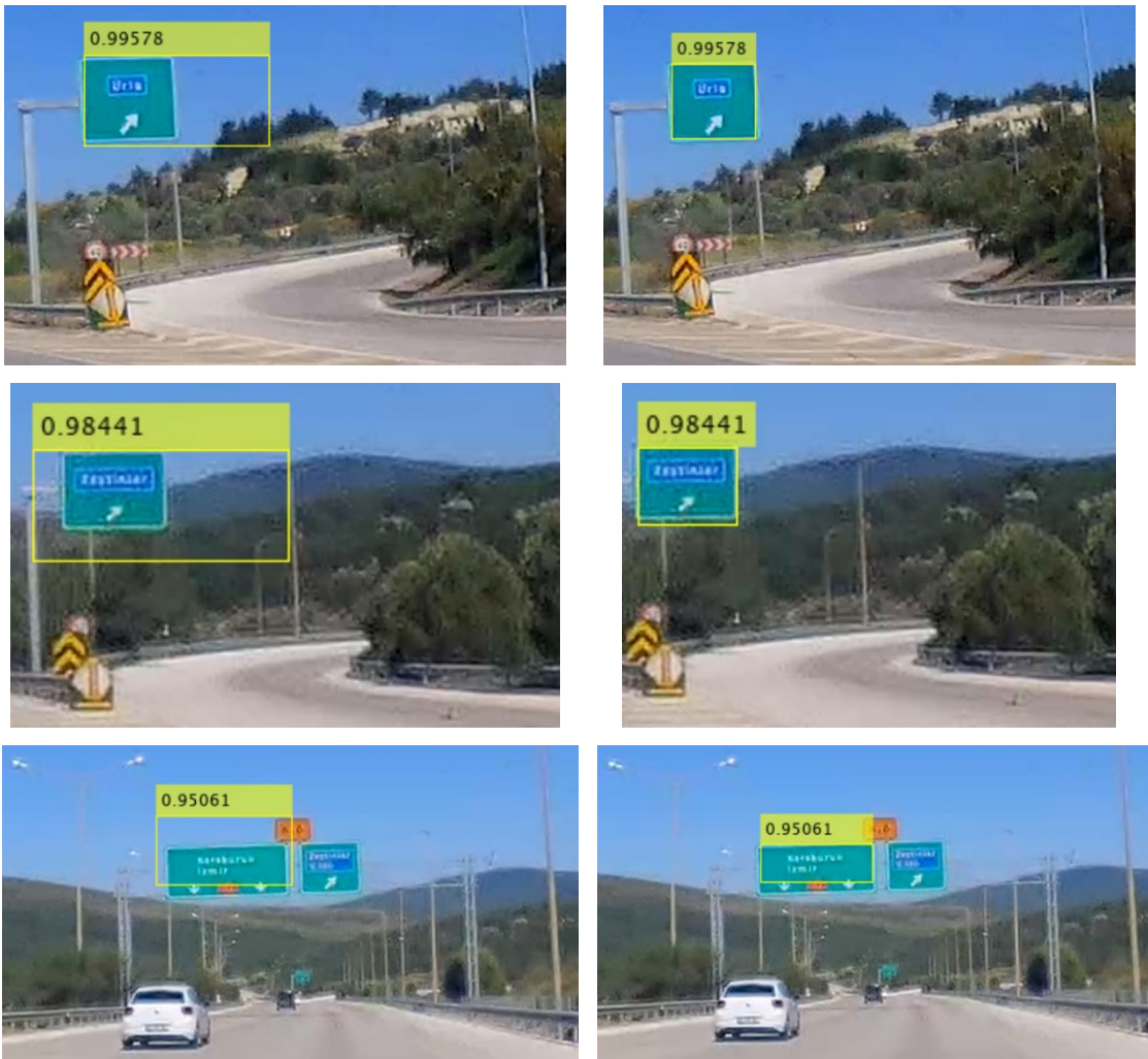
Figure 43. Localizations (left) can be improved (right) by a hybrid approach
