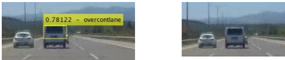
Figure 20. Most false positives can be corrected with location and size filters
