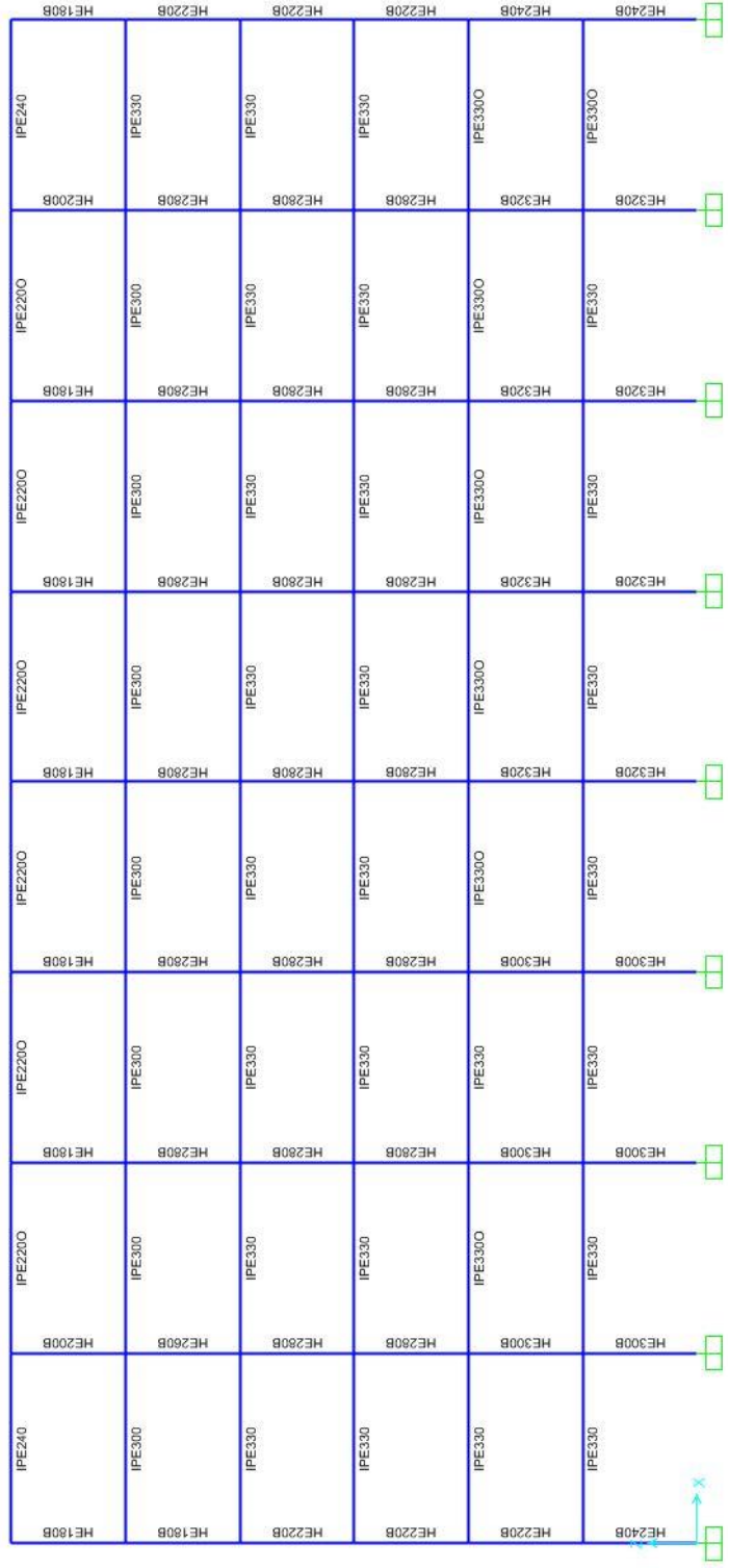
Figure A.34 Frame A86R8 member sections
