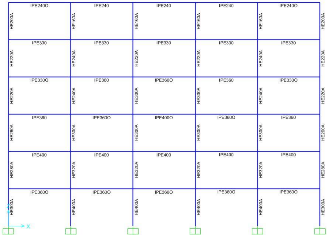
Figure A.15 Frame A56R4 member sections
