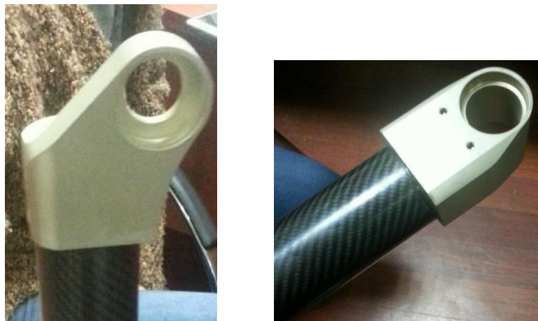
Figure A.1. A composite link for a high acceleration robot.
