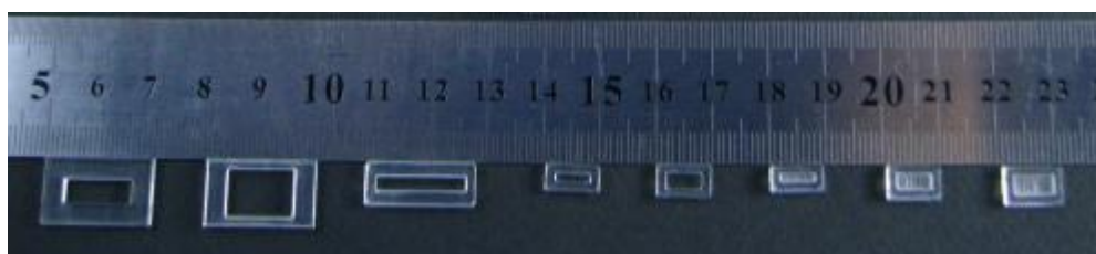
Figure 16. Digital image of fabricated PMMA substrates
