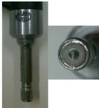
Figure 2.8.: The single-hole research injector. (Source: Cavicchi et al. [44] )
