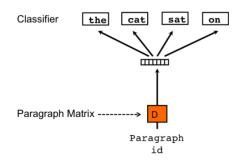
Figure 2.4. The DBOW network model
