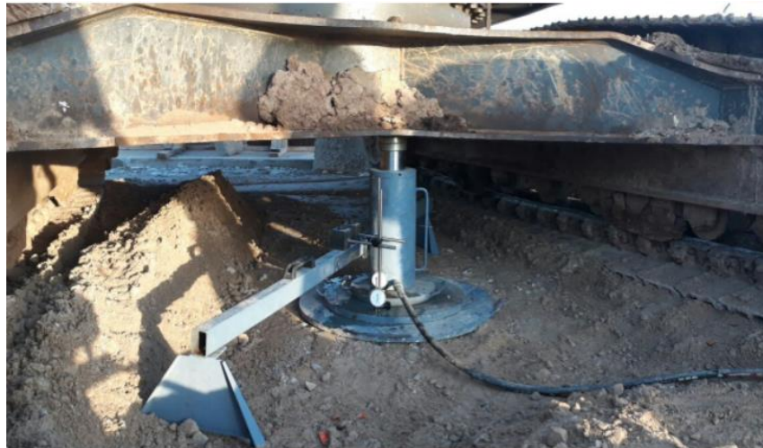
Figure 3.12. Plate Load Test in The Geothermal Project
