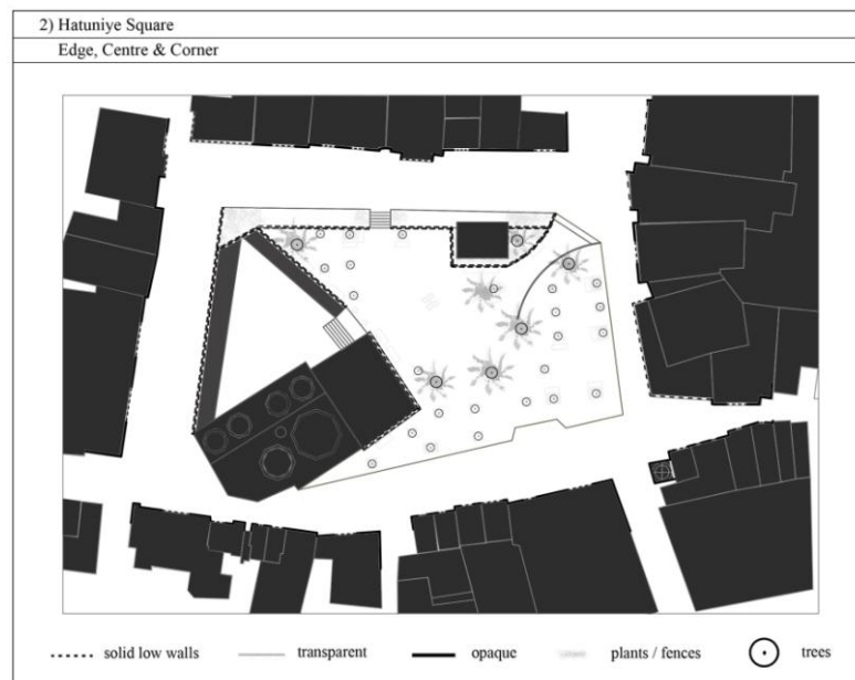
Figure 3.51: Surface qualities of surrounding walls in Hatuniye Square
