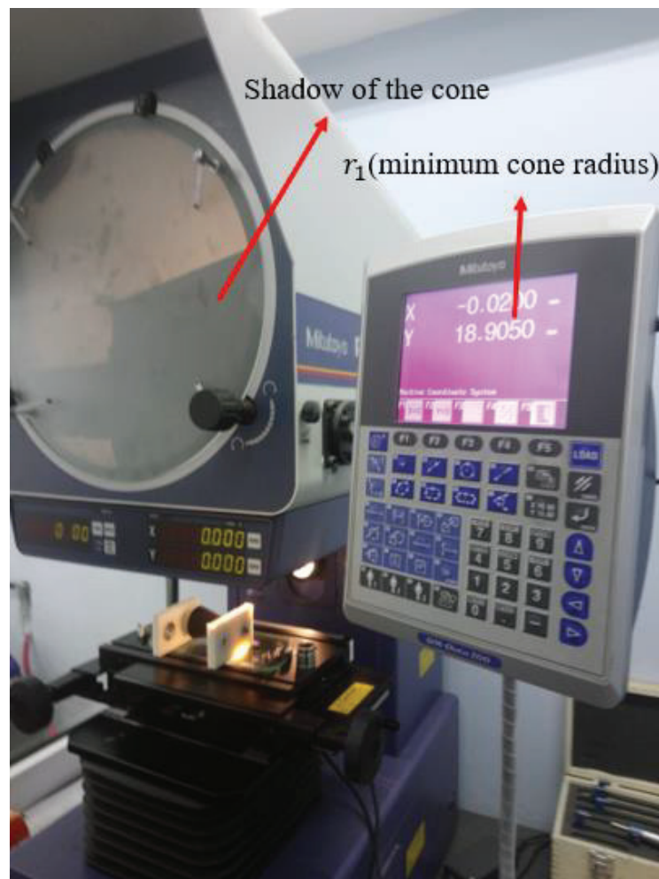
Figure 6.4. The measurement of the covered cone via profile projector machine
