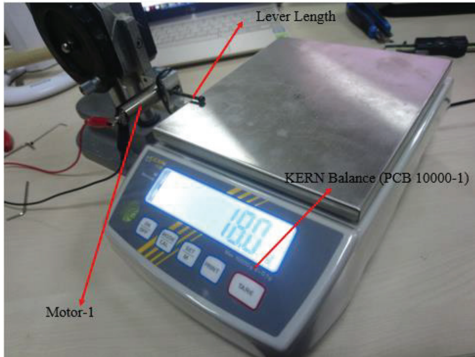
Figure 6.7. The torque constant validation setup of the Motor-1
