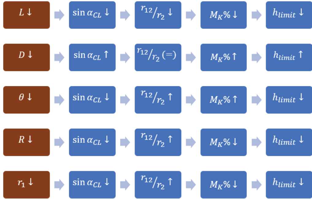
Figure 5.12. The flowchart for the effect of design parameters on the iteration results
