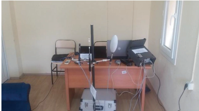
Figure 5.9. The PMV sensor used for measuring the PMV (Source: INNOVA, 2018)
