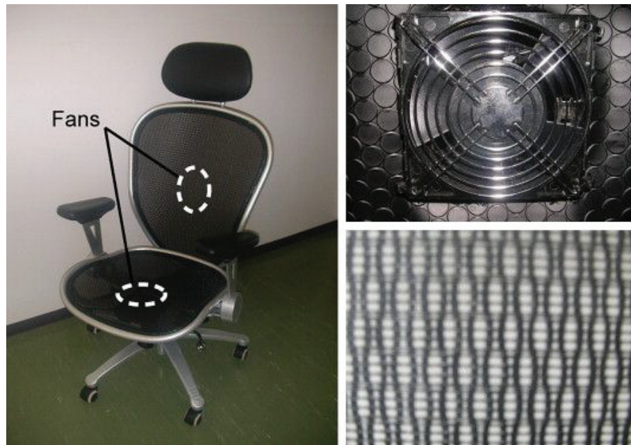
Figure 4.11. Personalized thermal comfort controller as a chair (Source: Watanabe et al., 2009)
