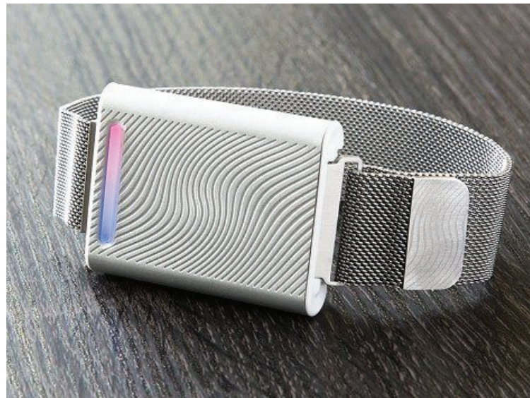
Figure 4.19. Personal wristband thermostat (Source: Embrlabs, 2018)
