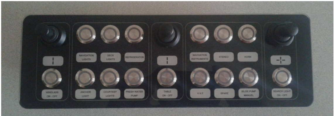
Figure 3.43. Northstar Orion 9 electronic control switches
