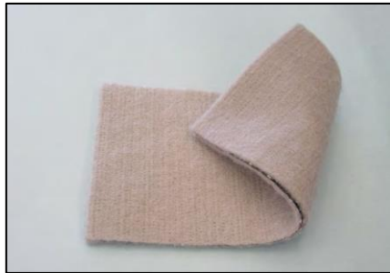
Figure 4.9 A Double-Sided Geocomposite Geomembrane
