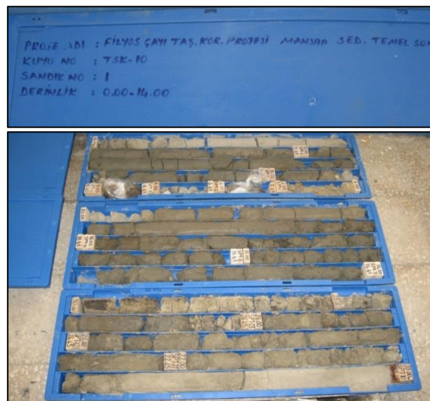
Figure A.7 Sample drilling well of TSK-10 at 758.18 m
