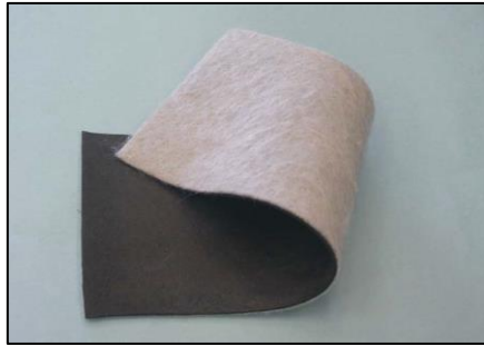
Figure 4.8 Single-Sided Geocomposite Geomembrane.
