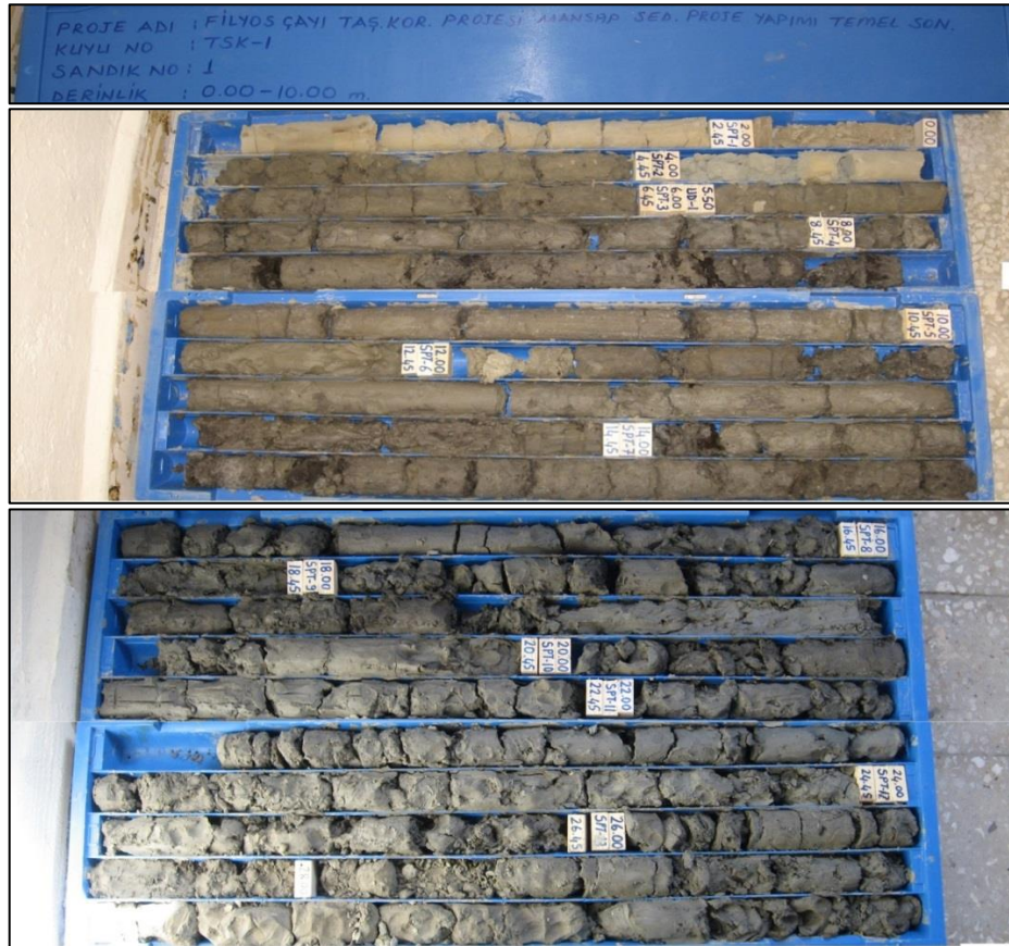
Figure 6.3 Sample drilling well of TSK-1 at 44.24 m
