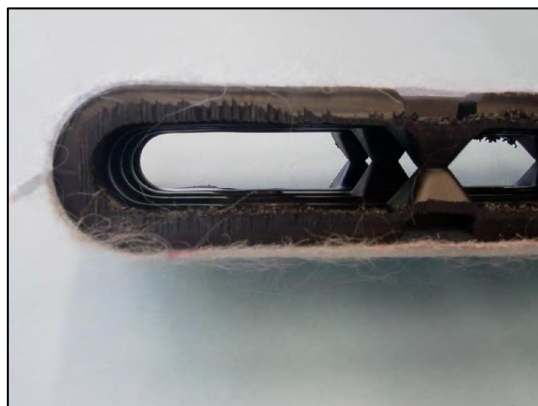
Figure 4.16 Photograph showing a close-up view of a portion of the geocomposite drain
