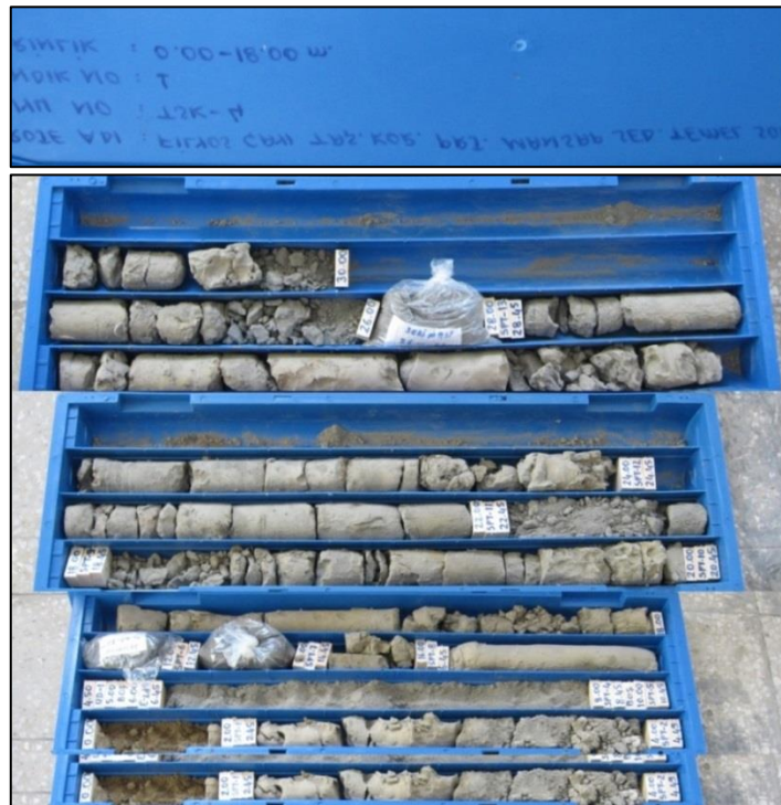
Figure A.3 Sample drilling well of TSK-4 at 1513.22 m
