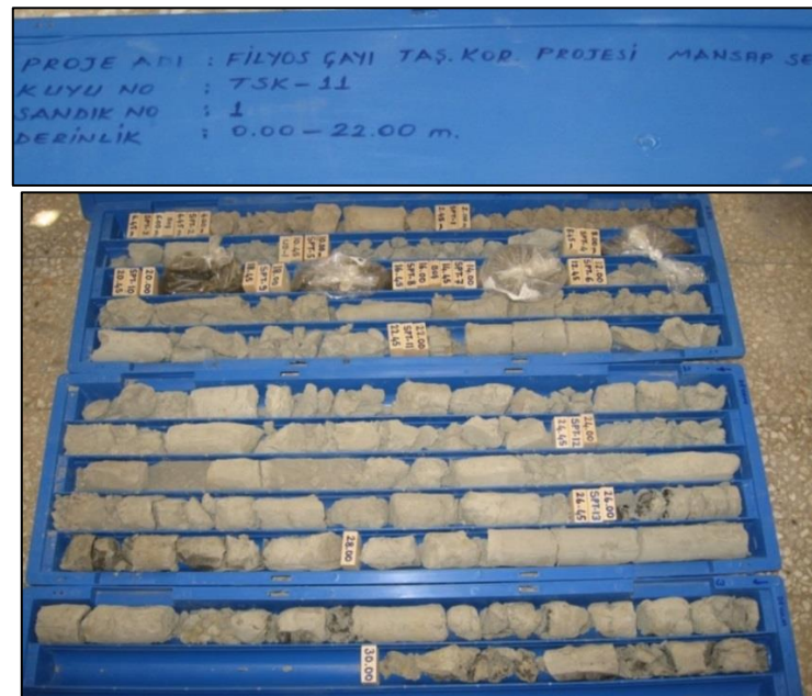
Figure A.8 Sample drilling well of TSK-11 at 1256.4 m
