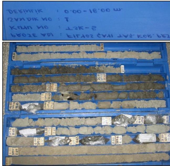
Figure A.4 Sample drilling well of TSK-5 at 2005.66 m
