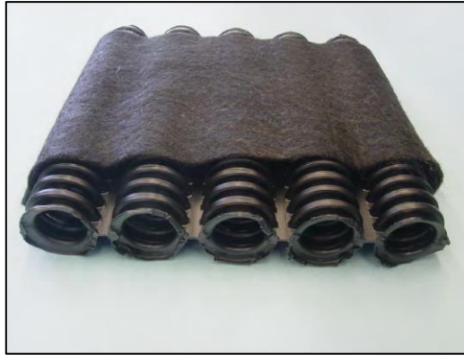
Figure 4.14 Geocomposite drain formed by enclosing a row of perforated geopipes inside a geotextile tube.
