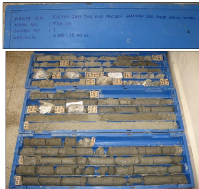
Figure A.10. Sample drilling well of TSK-13 at 2327.64 m
