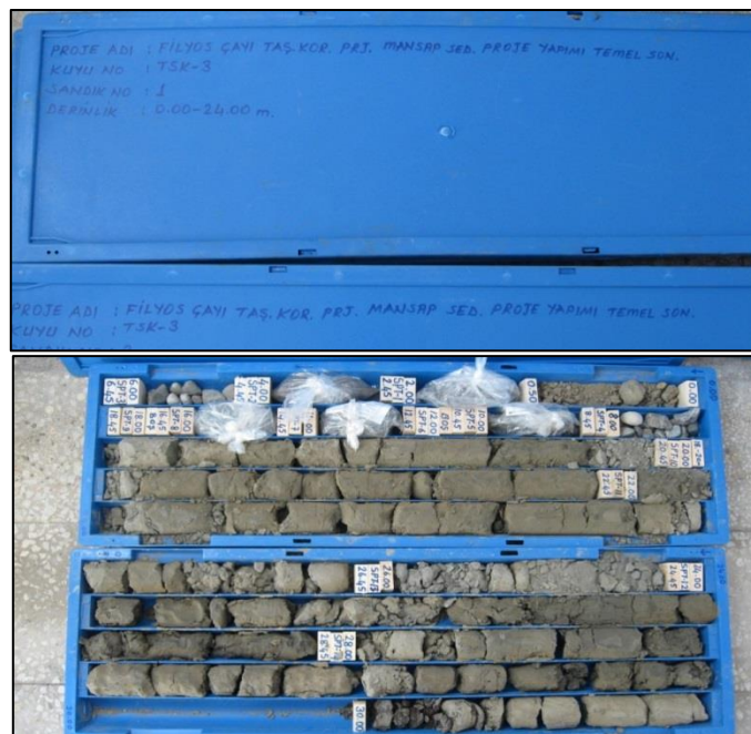
Figure A.2 Sample drilling well of TSK-3 at 1010.63 m
