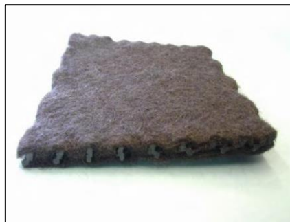
Figure 4.10 Geocomposite Geonet Drain
