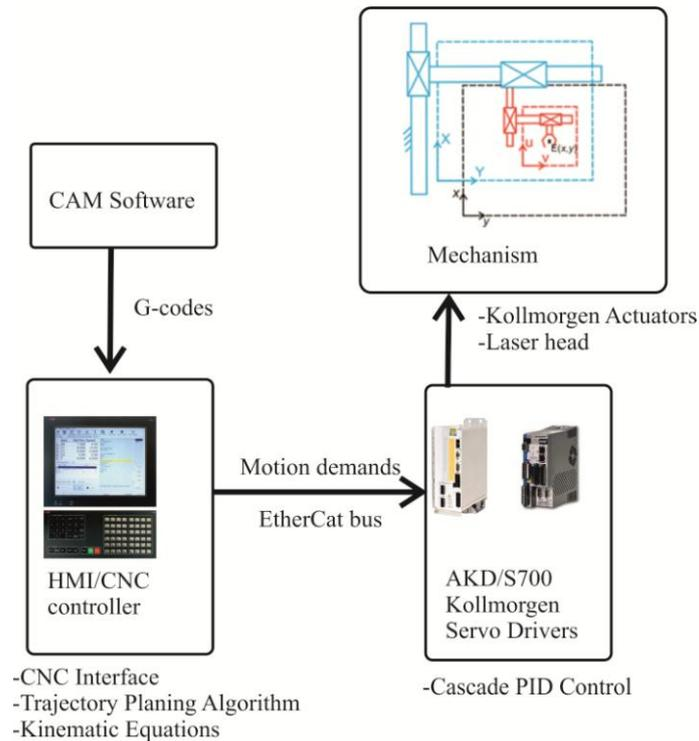
Figure 5. Hardware description of the control.
