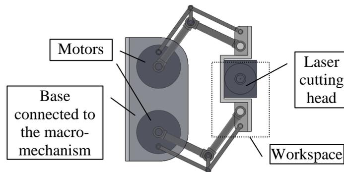
Figure 1. Micro-mechanism.
