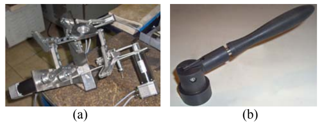
Fig. 29. Assembled (a) translation mechanism, (b) orientation mechanism
