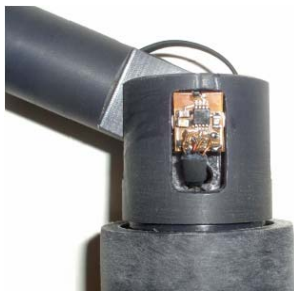
Fig. 31. Integration of the miniaturize position sensors
