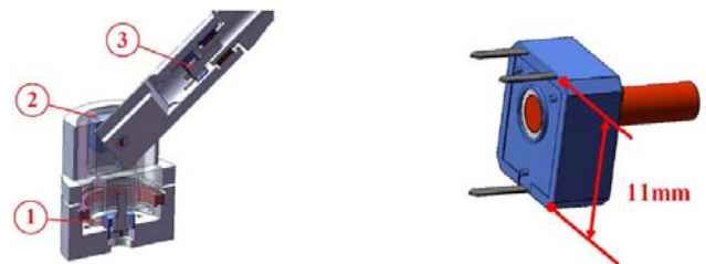
Fig. 23. Position sensors: (a) Location of the sensors, (b) Dimensions
