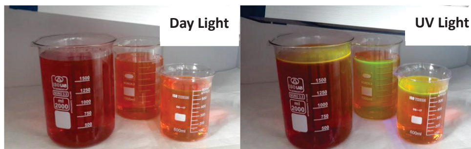
Figure 5.6. Images of TGA capped CdTe nanocrystals which are synthesized in 500 ml, 1000 ml and 2000 ml reaction vessels of high volume reactor.
