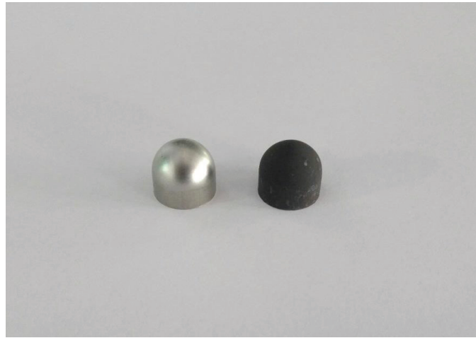
Figure 5.1. Specimens before and after heat treatment operation.
