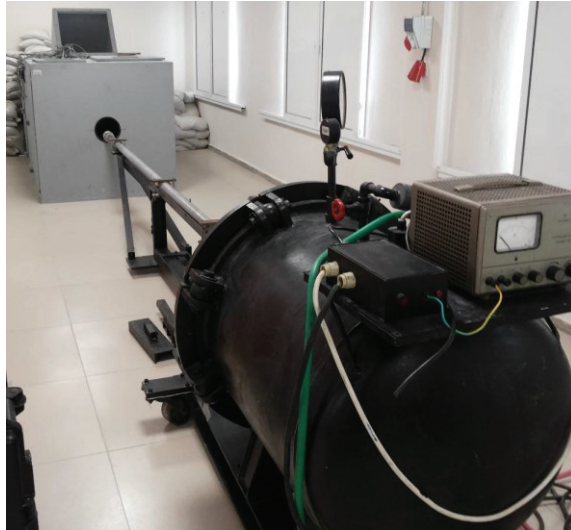
Figure 7.2. Ballistic test chamber of IZTECH.
