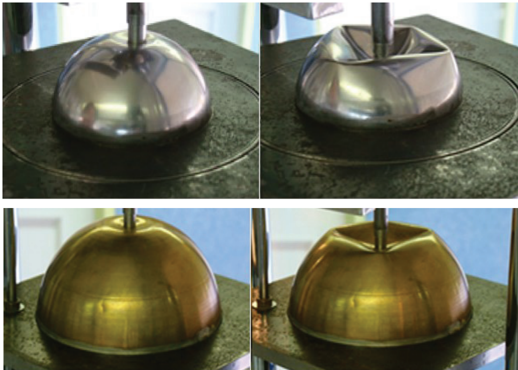
Figure 2.7. Progress of deformation on steel and bronze shells (Source: Amiri & Rasheed, 2012).
