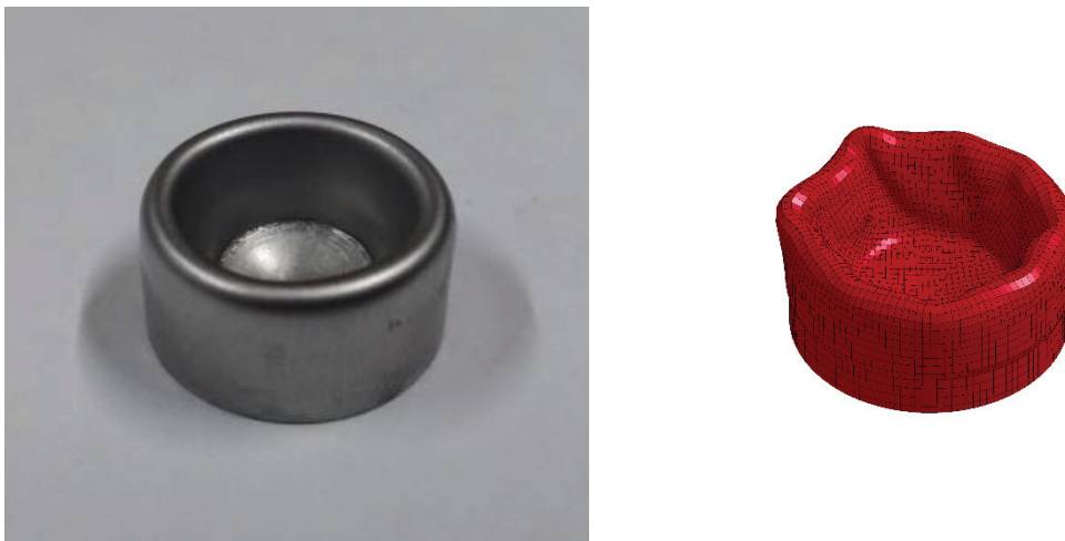
Figure 4.36. Comparison of experimental and numerical deformation of R75t05 core structure against blunt tipped indenter ( 1.3 \text{ mm.s}^{-1} ).
