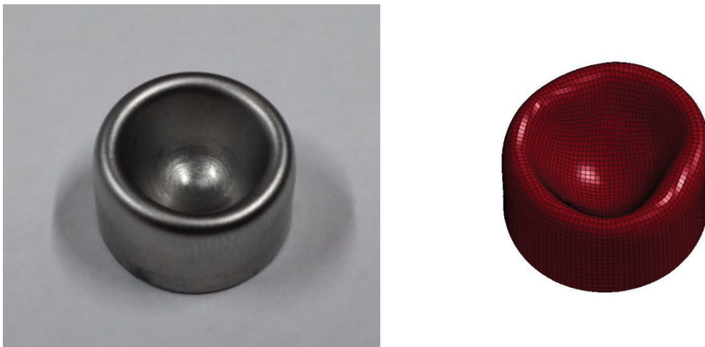
Figure 4.39. Comparison of experimental and numerical deformation of R75t05 core structure against hemispherical tipped indenter ( 1.3 \text{ mm.s}^{-1} ).
