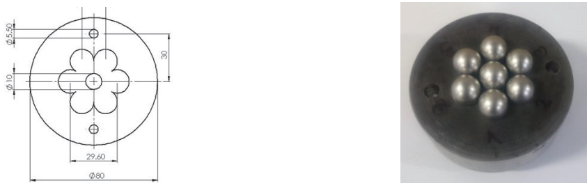
Figure 6.1. Specimen fixture used in experimental study and actual image captured before tests.
