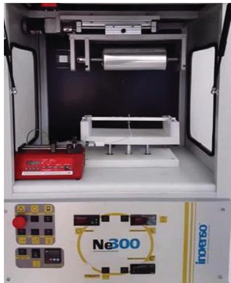
Figure 2.1. Electrospinning device (Inovenso NE300)
