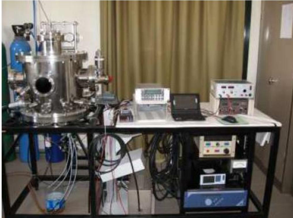
Figure 5. 2. Picture of magnetron sputtering system for deposition of Zn(O,S), ZnO and AZO layers.
