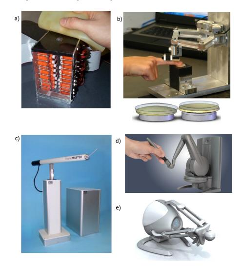
Figure 1.2. Tactile devices: a)Tactile pin array (Source: Wagner et al. (2002)). b)T-Pad tactile texture (Source: Winfield et al. (2007)). Kinesthetic devices: c)Haptic master 3DoF force reflecting haptic device (Source: Lab (2018)).
