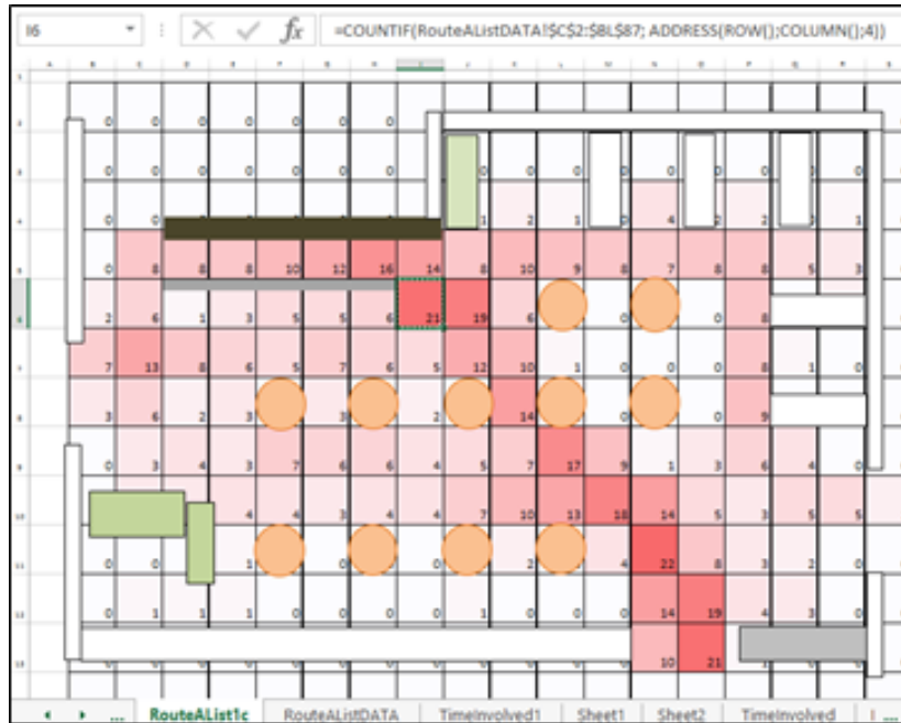
Figure 36. Plan Layout navigation density computed on cell resolution of 1 m 2 IEU Campus FFA Café
