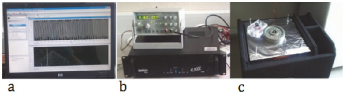
Figure 2.2. LMMS generating device. (a) View of the signal. (b) signal generator (top) and amplifier (bottom) (c) delivery of the signal to the culture plate via speaker.
