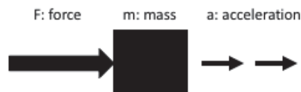
Figure 1.6. Force creates acceleration on constant mass.
