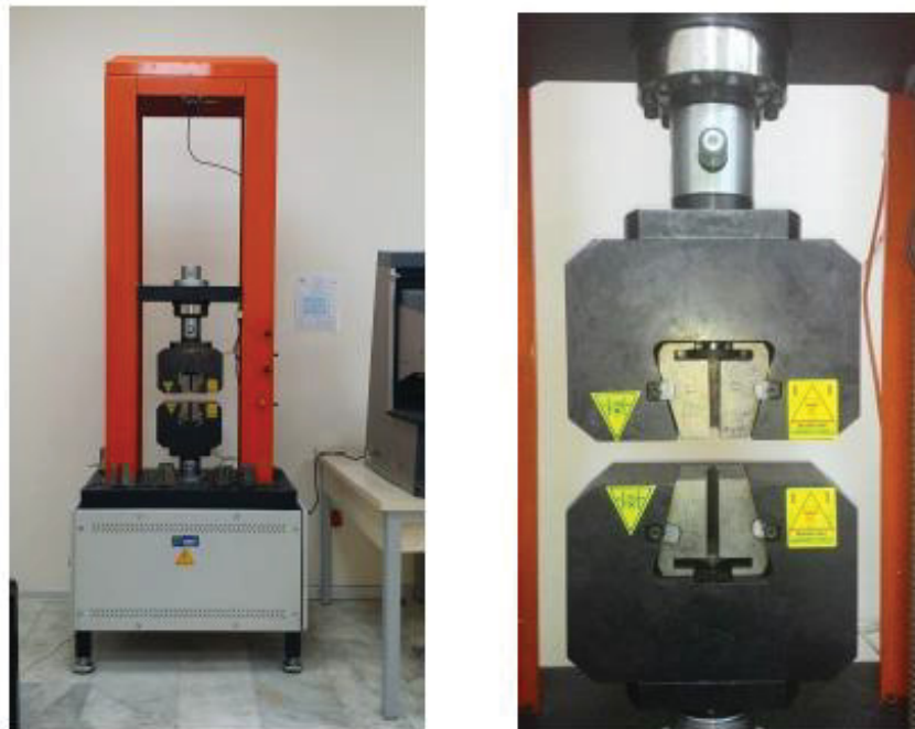
Figure 2.2. Tension test equipment (hydraulic tensile testing machine) (Source: NDE Research center)
