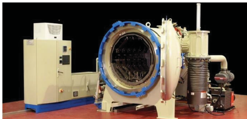
Figure 2.33. The commerical vacuum brazing furnace (Source: Peter Steege, 2015)
