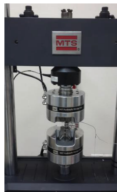
Figure 2.16. Hydraulic – axial fatigue test machine (Source: IYTE – ME, 2017)
