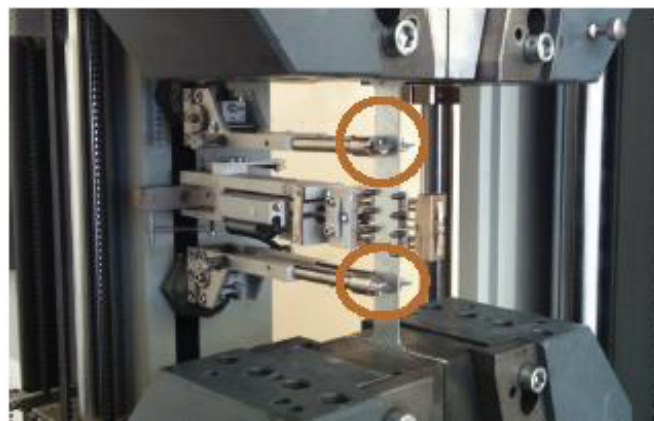
Figure 3.24. Macro extensometer (Source: Atılım University, 2016)
