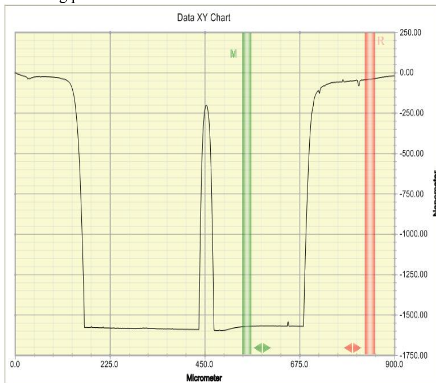
Figure 3.29 Surface analysis of the final structure in Fig. 3.28
