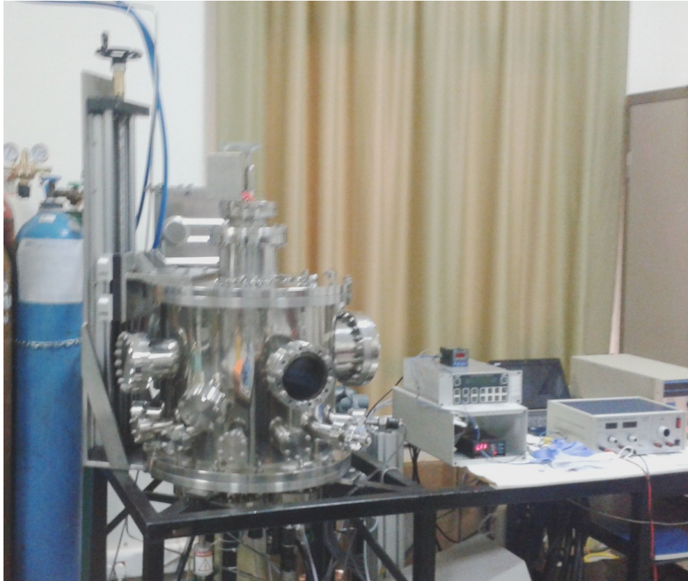
Figure 2.9 The figure shows the DC sputtering system in our laboratory which is used for thin film production
