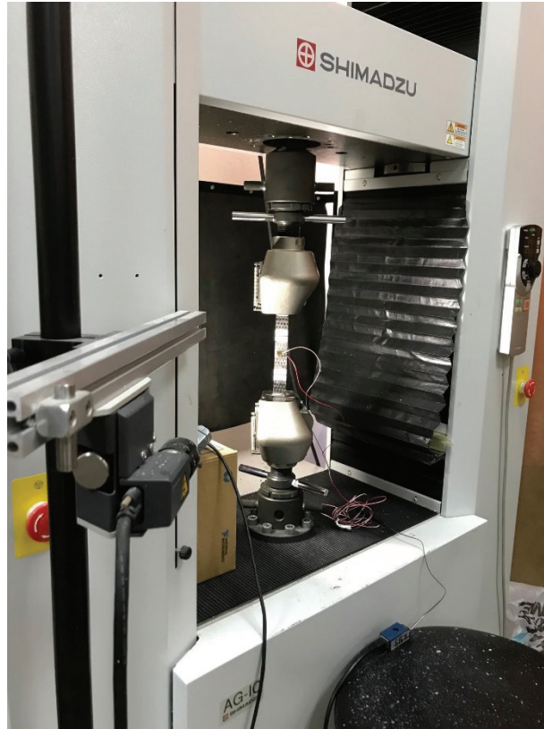
Figure 8.9. The representation of the Poisson's ratio test
