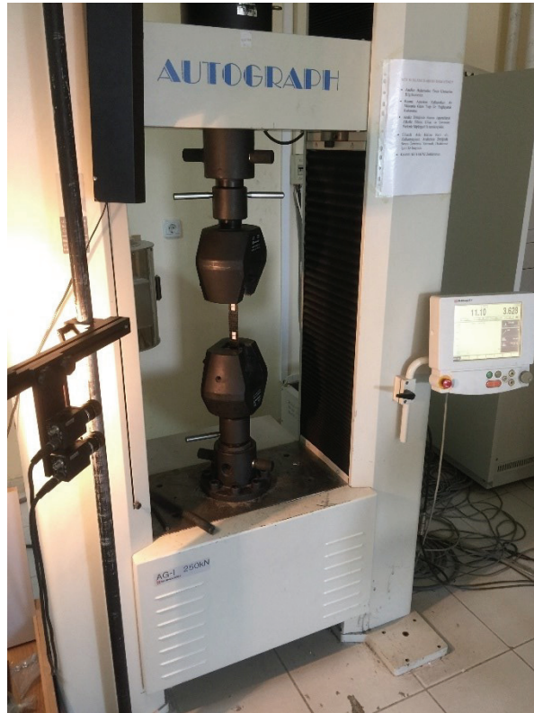
Figure 8.4. Shimadzu AG1 250 kN mechanical testing machine
