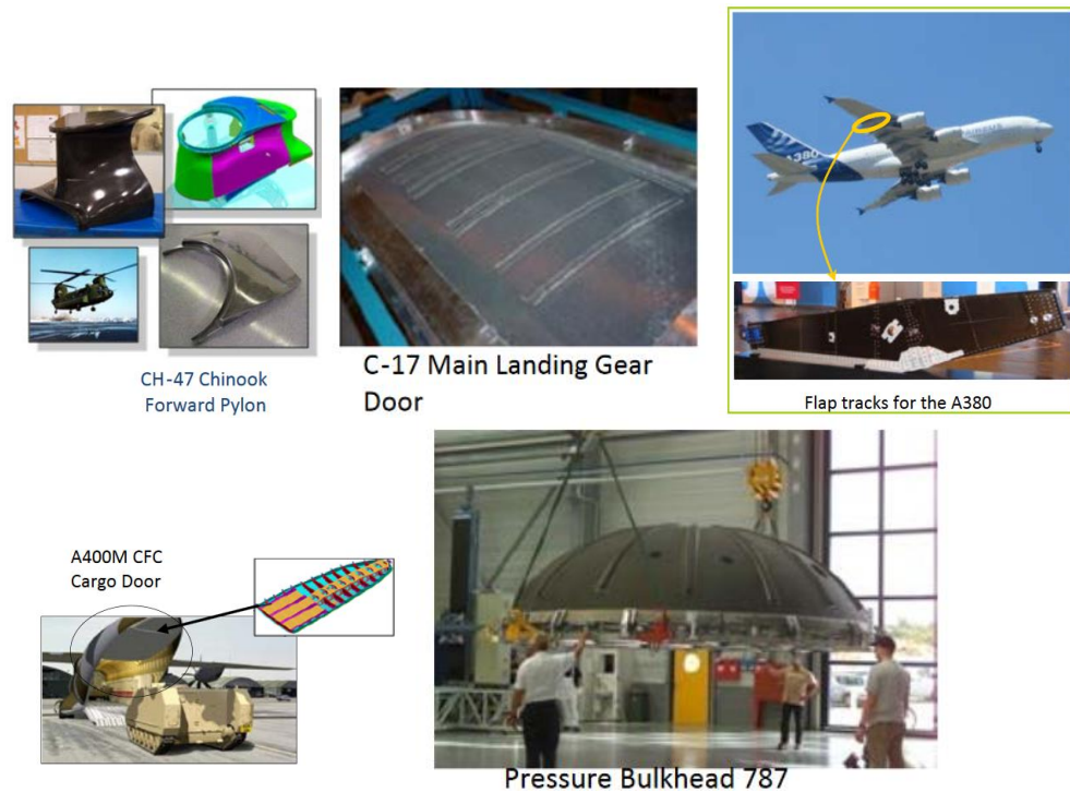
Figure 2.1.12. Recent applications of VaRTM method for aerospace component production [35].
