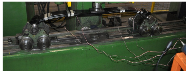
Figure 5. Steel leaf spring strain gauge measurement results
